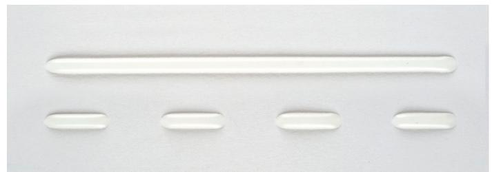
Instead of a single open/close cycle, the adhesive applicator now cycles 4 times in the same 2-inch distance.
